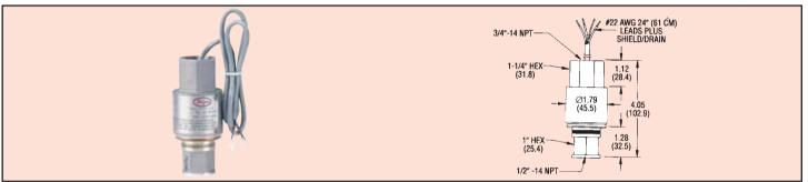
The Series 636 Pressure Transmitter is a low cost, fixed range, stainless steel transmitter with ±0.30% accuracy. It is designed to continuously measure pressure for years in even the toughest environmental and media conditions, Select from 4 ranges to 0-300 psig (0-20 bar) with choice of 4-20 mA output (model 636) or 1-5 VDC output (model 636LP). Transmitters are explosionproof, (FM approved) and meet NACE standards for offshore applications.
