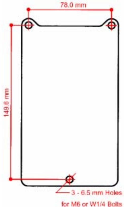
3. Due to the space is very small that is impossible to use wrench. Therefore, to use female expansion bolts on the wall or tap female screws on the steel plate and use external screw (male bolts) that can use the screw driver to install the gas detector and solve spacing problems. M6 sizes of bolts have a good tolerance than W1/4.
